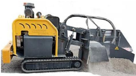
**TRANCHEUSE A FIBRE OPTIQUE FIBER 630**
